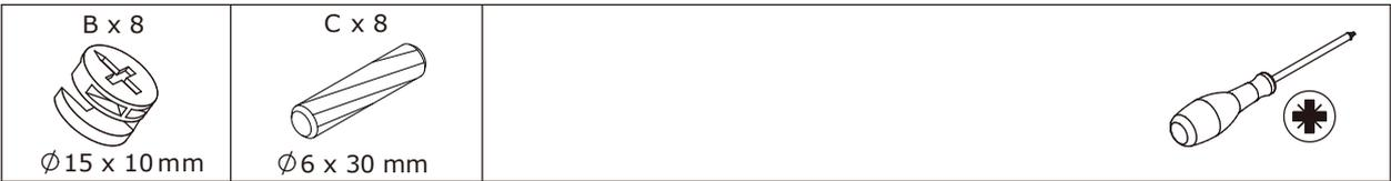
Cover plate 1 to plate 2,3,4,5 using wooden dowel(C) and turn cam lock(B) clockwise to tighten.
