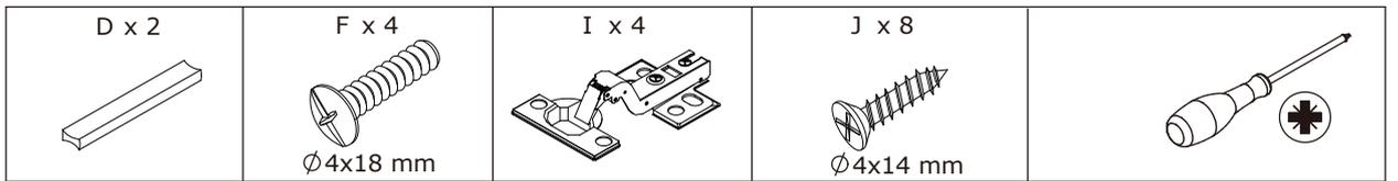
Fix hinge(I) to plate 6 and 7 respectively with screw(J) as shown. Please don't use an electric screwdriver or use force to rotate, may cause crack.
