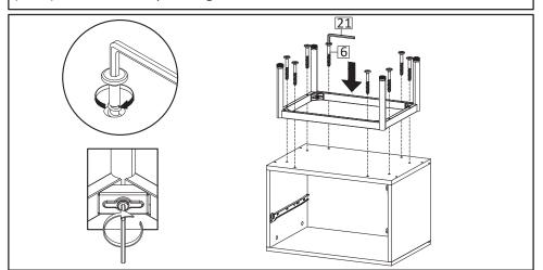
**STEP11**: Install assembled leg unit from Step 10 onto main assembled unit by inserting Screw (HW6). Tighten with Allen Key (HW21). Then tighten all the Screw on all corners of assembled leg.
