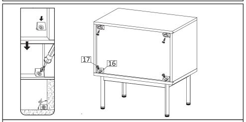
**STEP12**: Use Wedge (HW16), Screw M3.5x15.5mm (HW17) to tighten the back of night stand by using screwdriver. Please align the top board and bottom board in  $90^{\circ}$  position against the side board, before securing the wedges (HW16)
