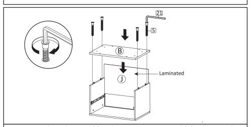
**STEP8**: Attach Back Board (J) and Insert Bottom Board (B), secure with Screw M7x50mm (HW5), tighten screws using Allen Key (HW21).
