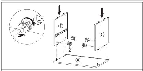
**STEP7**: Attach Side Board Left (C) and Side Board Right (D) into Top Board (A). Secure with Camlock Big (HW2) and tighten it using screwdriver.
