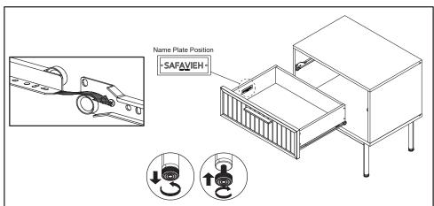
**STEP13**: Hold the sides of drawer, position the wheel of Drawer Runner at drawer back and the wheel of Drawer Runner at side boards, according to the image. Slide in the drawer into the night stand.
