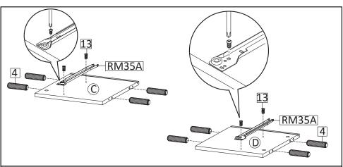
**STEP6**: Insert Dowel Big (HW4) into Side Board Left (C) and Side Board Right (D). Continue with securing part of the Drawer Runner (HW RM35A) into position as the above image, using screw M6x10.5mm (HW13).
