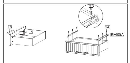
**STEP3**: Use Screw M4x22mm (HW19) to attach Handle (HW18) to the Front Drawer. Install the Drawer Runner (HW RM35A) into position as shown in picture. Secure with screws M3.5x13mm (HW14).
