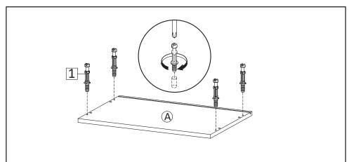
STEP5: Insert Cambolt (HW1) into Top Board (A).
