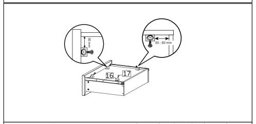
**STEP4**: Insert the Screw M3.5x15.5mm (HW17) and Wedge (HW16) into the bottom of the drawer according to the picture.
