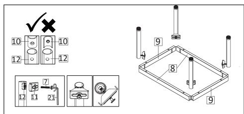
**STEP9**: Insert Support Corner Brace (HW10) and place it inside Leg (HW12) tube.Insert Screw (H7) into the hole of Corner Brace (HW11). Screw in slightly just enough to grip Leg (HW12) with Support Corner Brace (HW10) inside. Do not tighten. Arrange Support Metal Leg 1 (HW8) & Support Metal Leg 2 (HW9) on the floor as per image.
