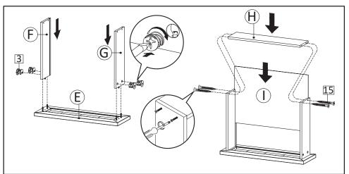
**STEP2**: Combine Side Drawers (F&G) into Front Drawer (E) then tighten Camlock Small (HW3) using screwdriver.Insert Bottom Drawer (I) with laminated face facing upward then put Back Drawer (H) and secure with Screw M8x39mm (HW15).
