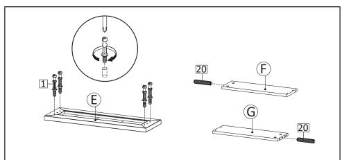
**STEP1**: Insert Cambolt (HW1) into Front Drawer (E). Insert Dowel Small (HW20) into Side Drawers (F&G).
