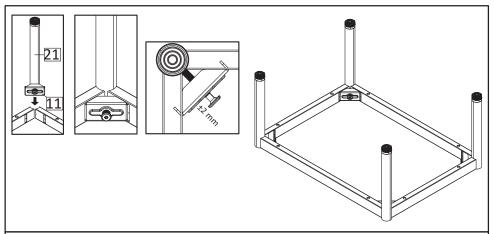
**STEP10**:Install the prepared Leg (HW12). Ensure the Corner Brace (HW11) hooks onto the hole of Support Metal Leg (HW8) and (HW9). Screw in just enough to grip the support using Allen Key (HW21). Do not fully tighten. Repeat for the other legs
