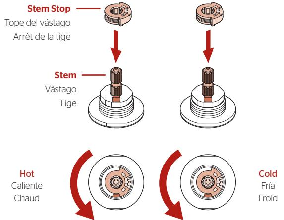
The Stem Stops can be inserted onto Stems in two different ways to accommodate preferred handle rotation.
