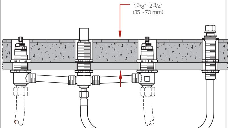
If deck thickness exceeds 1 3/8" (35 mm), Pfister™ Stem Extension Kit 974-375 must be used.
