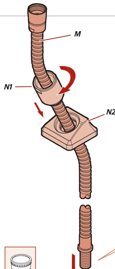
**Apply PTFE Plumber's Tape or Thread Sealant to all threaded fittings according to manufacturer's instructions.**
