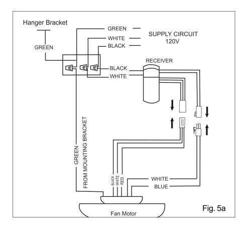
**NOTE:** Once ground wires are connected, carefully tuck all wires and marrettes into the metal box making sure that the wires are clear of the hemisphere and downrod when positioned in hemisphere and downrod when positioned in mounting bracket.
