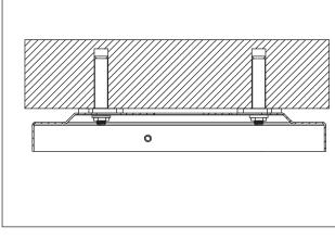
If installed on a wooden roof, use four wooden teeth screws.
