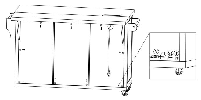
The Backboard Buckle T serves to assist in stabilizing the backboard structure. You can choose to install or not to install at will. This product can be used normally. When you choose to install it, you can directly screw in the screw T at the gap of the backboard.
