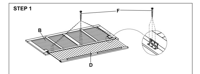
Attach the Top frame (B) to the back frame (D) on clean flat surface, secure with 5/8" screws (F) using screwdriver, position as shown.
