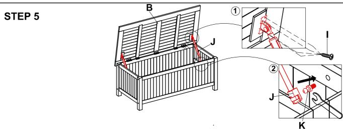
Attach lid support (J) into top frame (B), secure with 16 mm screws (I), as shown (figure 1). Next, attach lid nut (K) and lid bottom (J) to the right and left frame (A1 & A2), using wrench (figure 2).
