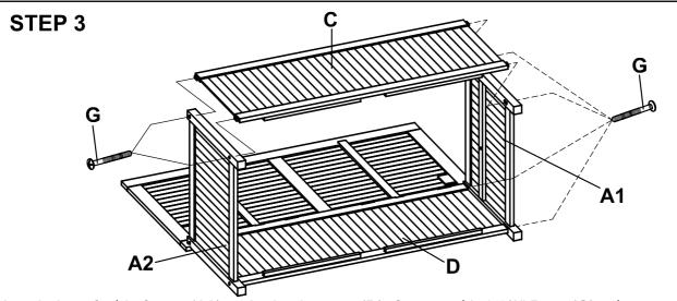
Attach the left side frame (A2) to the back apron (D). Secure with 1 1/2" Bolts (G) using screwdriver, do not fully tighten the bolts yet. Next, Attach front frame (C) to the Right side frame and left side frame (A1&A2) secure with 1 3/4" Bolts (G) using screwdriver
