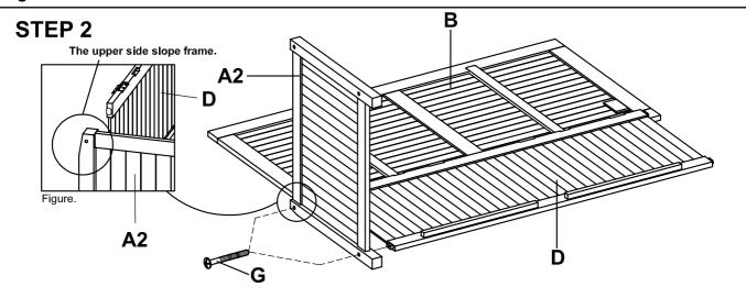
Attach the left side frame (A2) to the back apron (D). Secure with 1 3/4" Bolts (G) using screwdriver.
