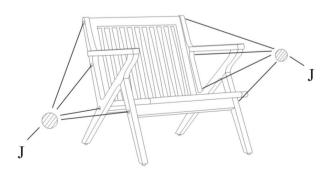
• step5 put the cover into each hole slightly
