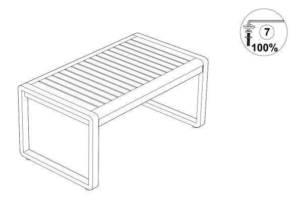
Put The table upright, then firmly tighten Bolts with Allen Key (7) to finish Table.
