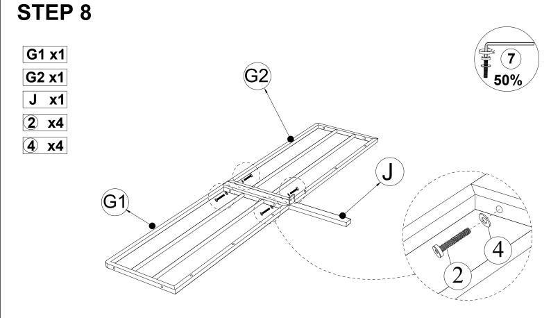
Connect Back Bench Frames (G1) & (G2) & Back Support Leg (J), tighten Bolt (2) & Flat Washer (4) & Allen Key (7).
