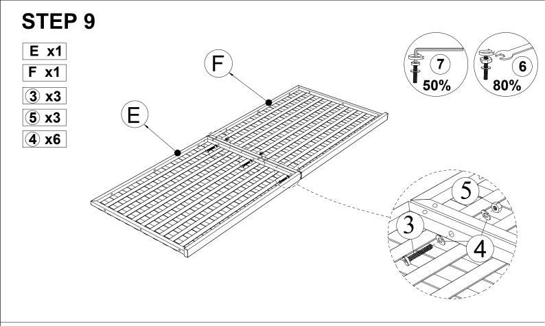
Connect Left Seat Bench (E) & Right Seat Bench (F), tighten Bolt (3) & Flat Washer (4) & Nut (5) with Allen Key (7) & Key (6)
