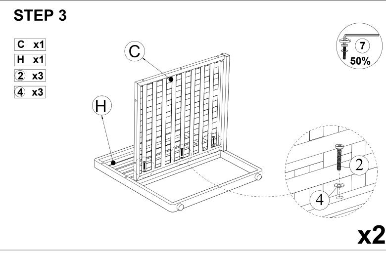
Connect Seat Chair Frame (C) & Left Armless (H), tighten Bolt (2) & Flat Washer (4) & Allen Key (7).
