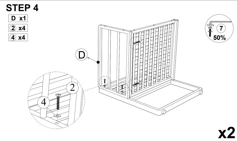
Connect The part from Step 3 & Back Chair Frame (D), tighten Bolt (2) & Flat Washer (4) with Allen Key (7).
