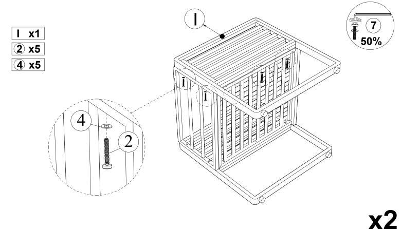
Connect The part from Step 4 & Right Armless (I), tighten Bolt (2) & Flat Washer (4) & Allen Key (7).
