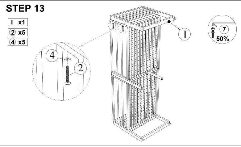
Connect The part from Step 12 & Right Armless (I), tighten Bolt (2) & Flat Washer (4) & Allen Key (7).
