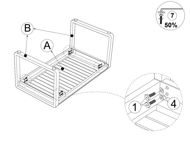
Connect Leg Table (B) & Top Table (A), tighten Bolt (1) & flat washer (4) with Allen Key (7).
