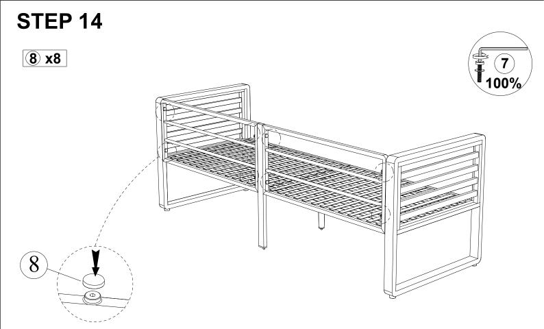
Put the Bench upright, firmly tighten Bolts with Allen Key (7), push Plastic Cover (8)
