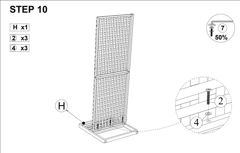
Connect The part from Step 9 & Left Armless (H), tighten Bolt (2) & Flat Washer (4) & Allen Key (7).
