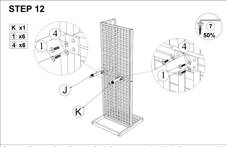
Connect The part from Step 11, Back Support Leg (J), Middle Support Leg (K), tighten Bolt (1) & Flat Washer (4) & Allen Key (7).
