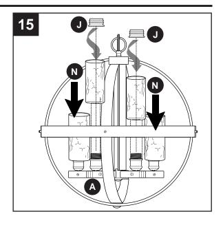
Install four 60-watt max. standard-base incandescent bulbs (not included) or CFL/LED equivalent.
