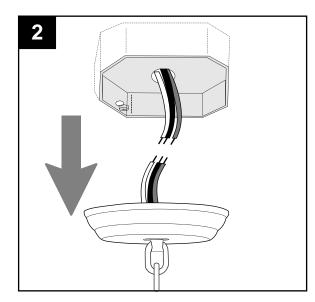
Attach mounting strap (C) to outlet box (not included) using existing washers and outlet box screws or the machine screws (BB). NOTE: If the outlet box screws required for your outlet box are of a different size than the machine screws (BB), consult a licensed electrician before proceeding.
