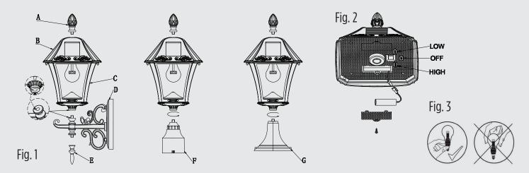
1. Remove the Top (B) from Body part (C) by unscrewing the 2 screw caps. Install the new GS Solar LED Light Bulb by turning it into the bulb socket located at the top of the light clockwise. Bulb needs to be installed before lamp is turned on.
