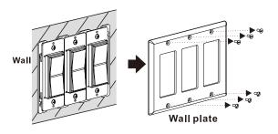
3-2. Uninstall the wall switch from the switch box by removing two screws from the switch box. (Keep these screws for step 3-5.)
