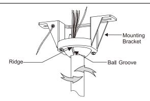
② Rotate fan so that the groove on the ball engages the ridge in the mounting bracket.
