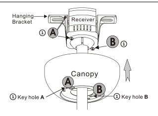
**Note:** Two screws are pre-installed on mounting bracket for canopy installation.
