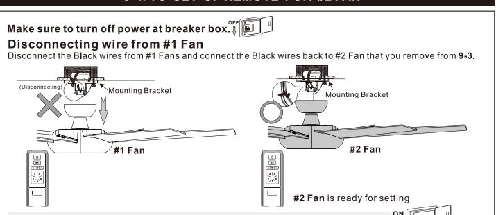
Turn on power at breaker box and #2 Fan is ready for setting.
