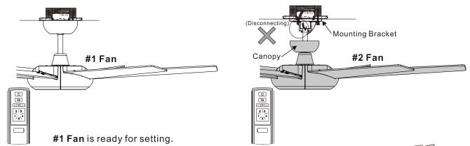
Turn on power at breaker box and #1 Fan is ready for pairing.
