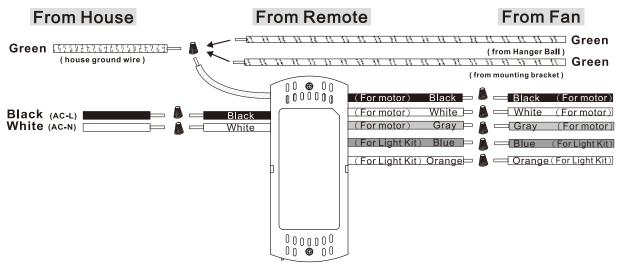
"Special note: All Green grounding wires, from <u>Hanger ball/Mounting bracket/Receiver</u>, must be well attached to House Ground/Earth to prevent flickering of LED."
