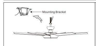
1 Lift fan assembly onto mounting bracket.
