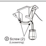
2 Loosen the screws at mounting bracket. Do not remove.
