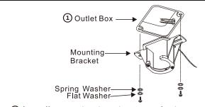
1 Install mounting bracket to outlet box on ceiling by using screws included with the outlet box and washers from the hardware bag.
