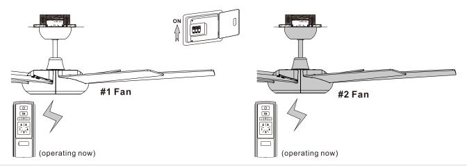
**NOTE:** For more than two fans, the same rules apply. Make sure only one fan at a time is connected to power when doing the Remote Setting. Already completed fans should be disconnected until all fans have completed the Remote Setting process.
