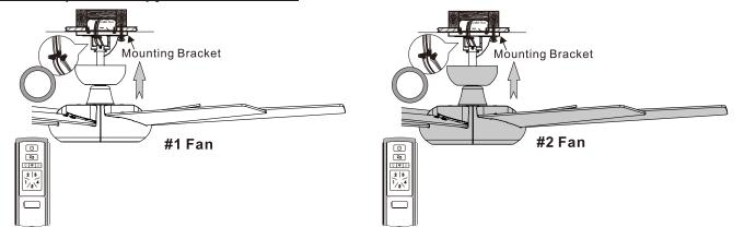
**9-6.** Switch on the main power and now each of these two fans are operated by its own remote individually.
