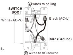
IMPORTANT: FAN'S REMOTE RECEIVER IS NOW DIRECTLY CONNECTED TO AC POWER. ON/OFF IS NOW OPERATED BY REMOTE TRANSMITTER.
