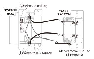
3-4. Connect the Black wire that goes to the ceiling box to the Black wire(s) from the AC source using the wirenuts provided.
