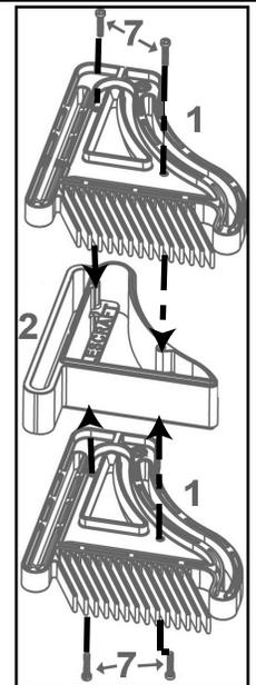
Also included is a second feather board and hardware necessary to run either dual feather boards, or a tandem stacked feather board. The tandem operation of the D/T FeatherBoard™ is ideal for thick material cutting operations.
