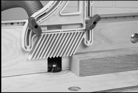
Set the first shortened feather to the top of the stock to ensure proper tension.
