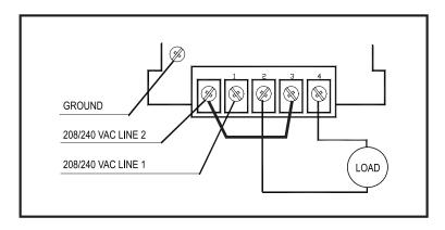
If you are using the 59104RWD with two loads, no jumper wire is needed and the unit should be wired as shown below.
