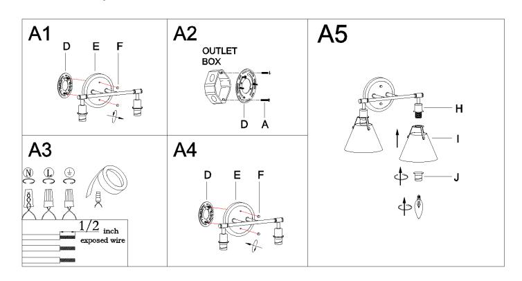
Step A1: Unscrew knob nuts (F) from back plate (E), then set them aside for later installation.
