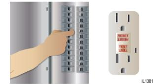
B. If pump does not run, check the GFCI or breaker panel switch to make it is in full operation.
