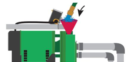
C. If the pump runs all the time, make sure the pump has been primed correctly. If pump is not holding the prime, inspect check valve, foot valve, and piping, then reprime.
