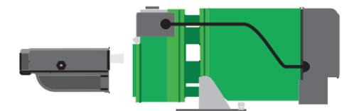
D. If the pump runs but won't shut off, check pressure switch.
