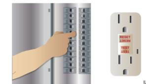
B. If pump does not run, check the GFCI or breaker panel switch to make it is in full operation.
