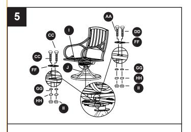
Once all connections are made, tighten CC,DD,FF,GG,HH, II with DD.
