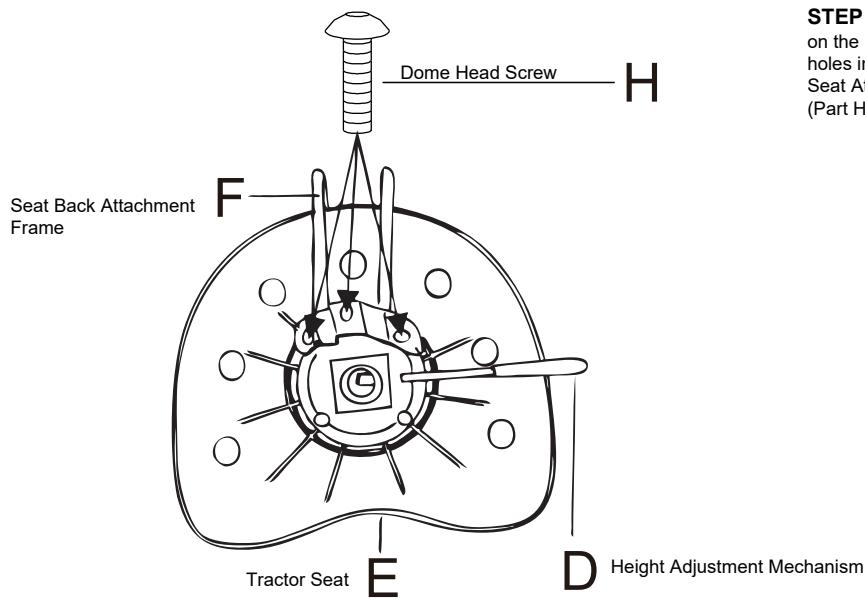
**STEP 3:** Place the Seat Back Attachment Frame (Part F) on the underside of the Tractor Seat (Part E) on top of the holes in the Height Adjustment Mechanism. Attach the Seat Attachment Bracket using (3) Dome Head Screws (Part H). Tighten with the Allen Wrench (Part I)
