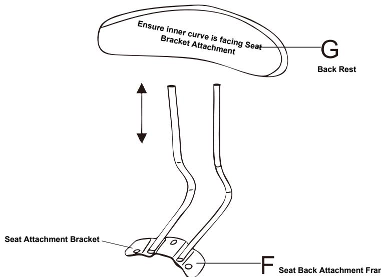
**STEP 2:** Push Seat Back (Part G) onto posts of Seat Back Attachment Frame (Part F).
