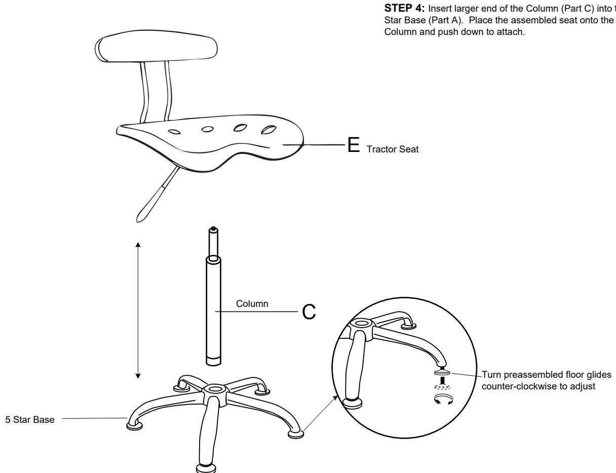
**STEP 4:** Insert larger end of the Column (Part C) into the 5 Star Base (Part A). Place the assembled seat onto the Column and push down to attach.
