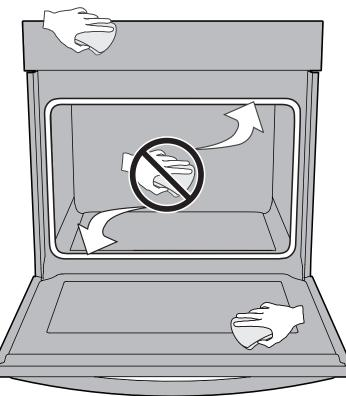
Figure 11: Do not clean oven door gasket
