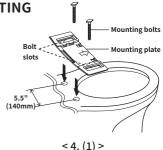
(2) INSERT MOUNTING BOLTS THROUGH THE BOLT SLOTS AND INTO THE BOLT HOLES IN THE TOILET.
