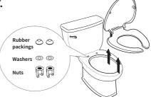
2. DRAIN TOILET WATER TANK COMPLETELY AFTER TURNING OFF THE WATER SUPPLY BY TURNING THE SHUT OFF VALVE CLOCKWISE.
