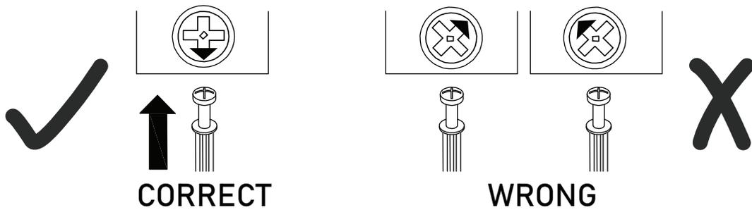
Quickfit head should be in the centre of the cam lock when the two panels are joined.
