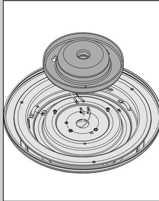
Connect the single-pin connectors from the LED assembly to the connectors from the fan. Connect the white wires together. Connect the blue and black wires together. Then, wrap keyhole slots around the screws and twist counterclockwise.
