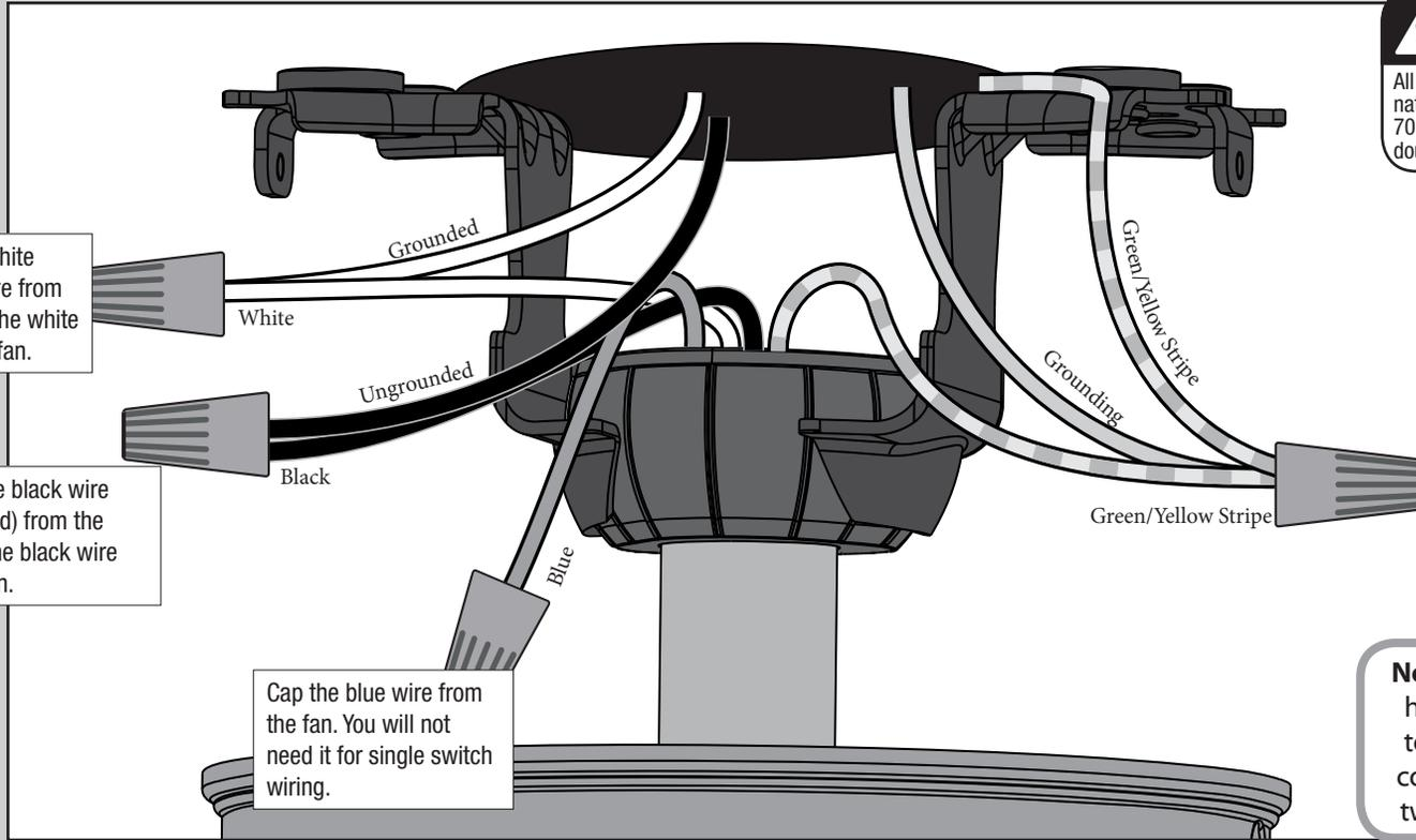
Connect the white (grounded) wire from the ceiling to the white wire from the fan.
