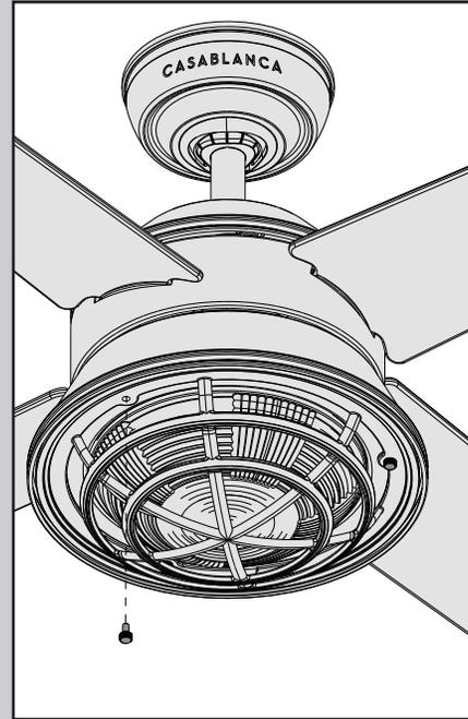
Attach the cage to the fan using the provided thumbscrews.
