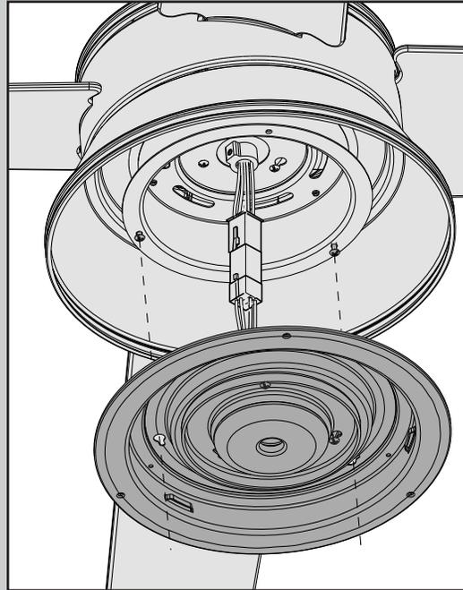
Connect the 9-pin wire connector coming from the fan to the connector coming from the electronics module on top of the lower switch housing. Make sure to line up the colored markings on the connectors. Then, wrap keyhole slots around the screws and twist clockwise.
