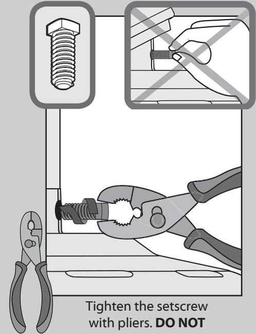
Tighten the setscrew with pliers. **DO NOT HAND TIGHTEN.**
