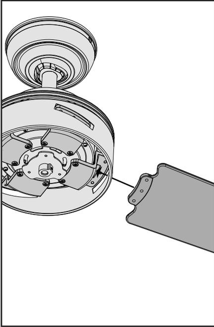
Insert a the blade through the slot. Align the screw holes in the blades with the screw holes in the on the blade ramp.
