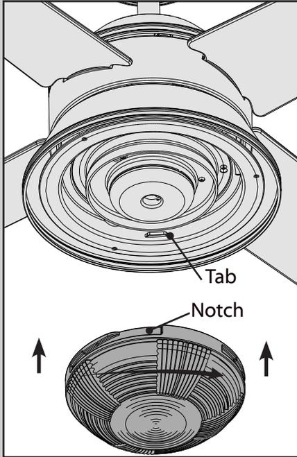
Position the notches in the outer rim of the globe so they line up with the three tabs on the inside rim of the housing. Carefully lift the globe up inside the housing as far as it will go, then rotate the globe clockwise until it is held tightly in place by the tabs.
