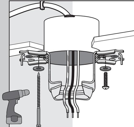
**Use wood screws** (included) when securing to support structure with approved electrical outlet box. Drill 9/64" pilot holes in support structure to aid in securing ceiling bracket with hardware found in the ★ hardware bag.
