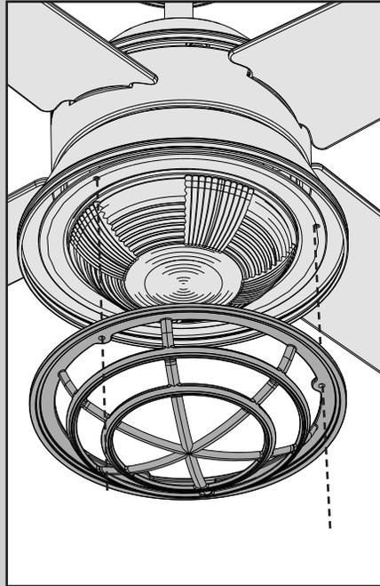
Lift the bottom cage. Align the screw holes in the cage with the screw holes in the lower switch housing.
