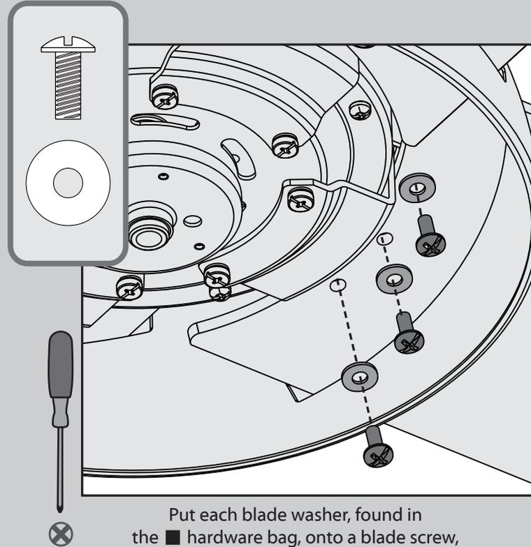
Put each blade washer, found in the ■ hardware bag, onto a blade screw, found in the ▲ hardware bag. Then secure each blade to the motor assembly using the blade screws and washers.
