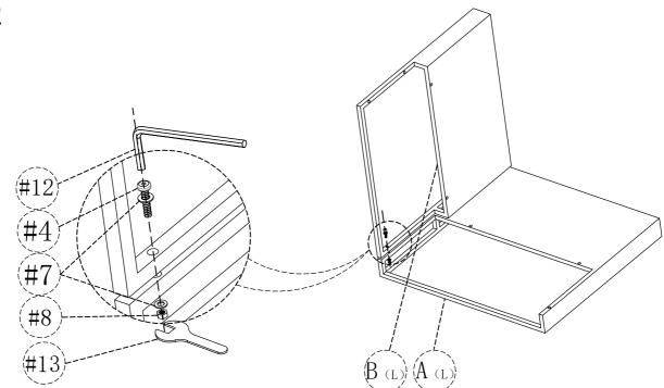
For this installation step, please tighten the screws by 80%
