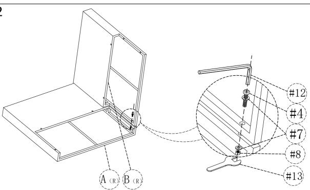
For this installation step, please tighten the screws by 80%
