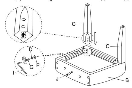
Take the Allen Wrench, and turn the bolts until the legs are secure. DO NOT TIGHTEN COMPLETELY. Stop when you feel you are adding force to tighten the bolt.
