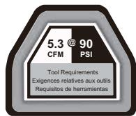
**IMPORTANT:** To operate correctly, this tool requires airflow that is at least 5.3 cubic feet per minute (CFM) at 90 pounds per square inch (PSI). Check the specifications of your air compressor to be sure that it can support both the minimum CFM and PSI required. An air hose may cause up to 15 PSI drop in pressure, so you may need to set the output higher to maintain the required pressure at the tool.
