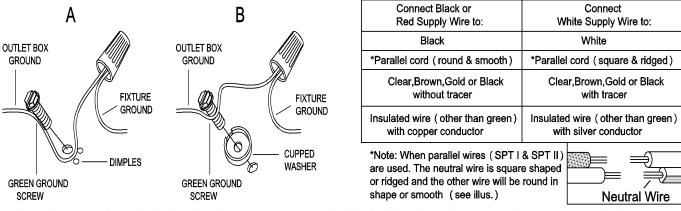
Twist wires together with plastic wire connector until tightly joined, and wrap each connector with approved electrical tape. Be sure that no wire strands are exposed and then carefully tuck all wires into the outlet box.
