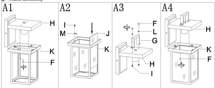
Step A1: Unscrew knob nuts (F) and remove iron frame (K) from cover (H).
