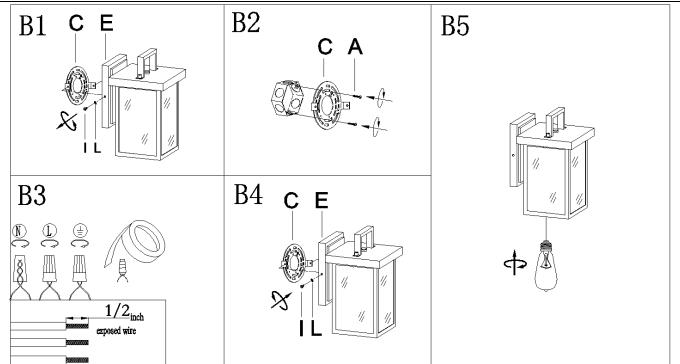
Step B1: Unscrew screws (I) and remove plastic washers (L) from mounting plate (C), then set aside for the following steps.
