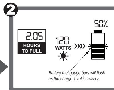
The intelligent LCD screen will show the solar icon, the input power and the battery charge level. (Press the DISPLAY button to turn off this screen if desired)
