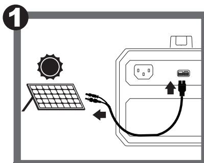
Connect your solar panel\* (200W max) to the Solar Input port in the back of your Battery Generator.
