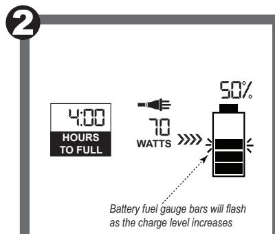
The intelligent display will show the AC icon, the input power and the battery charge level.
