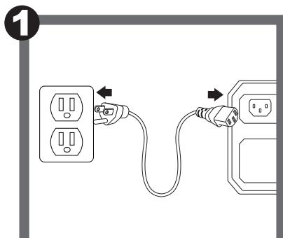
Plug the AC charging cord into the AC input on the back of your Battery Generator. Plug the other end of the cord into an AC outlet.
