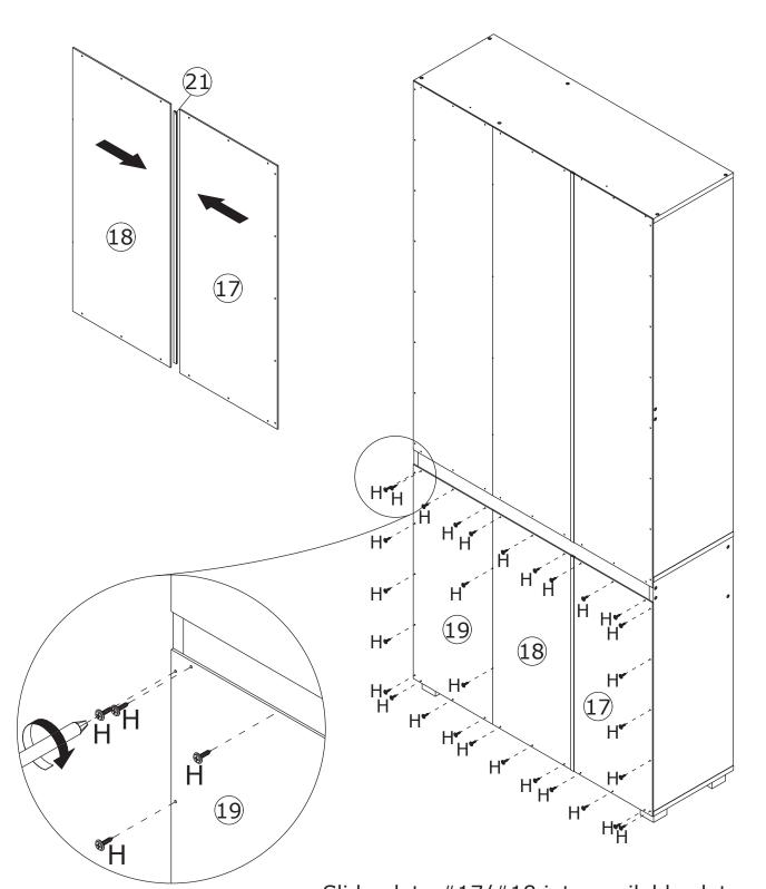
Slide plate #17/#18 into available slots of part #21, fix plate#17/#18/#19 to the component(assembled in step 12) using screw(H) as shown.
