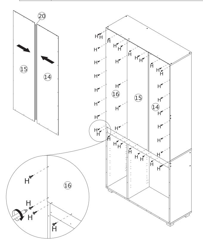
Slide plate #14/#15 into available slots of part #20, fix plate #14/#15/#16 to the component (assembled in step 11) using screw(H) as shown.
