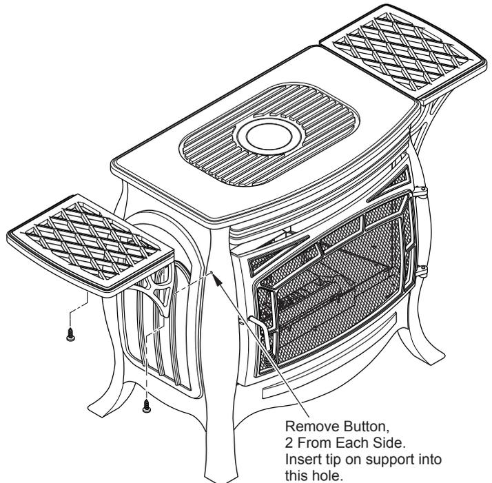
Remove Button, 2 From Each Side. Insert tip on support into this hole.
