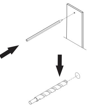
Use a Ø8mm drill bit to drill the wall.
