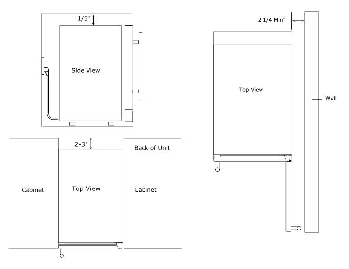
Units have a zero clearance for the door to open 90°, when installed adjacent to cabinets.
