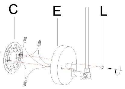
Tighten the pre-assembled hex nuts and back to step 7.
