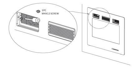
(Only for all models of style C which has no mesh for the air inlet.)
