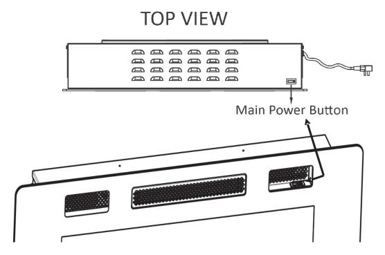
Note: Make sure the Main Power Switch is turned on before operating.
