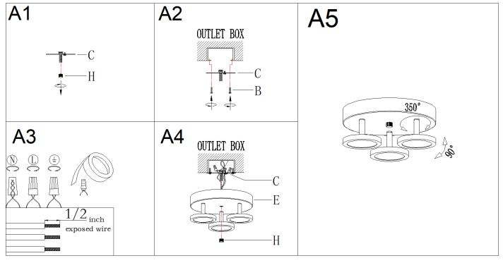
Step A1 » Unscrew cap nut (H) from single bar (C), then set them aside for later installation.
