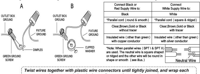
connector with approved electrical tape. Be sure that no wire strands are exposed and then carefully tuck all wires into the outlet box.
