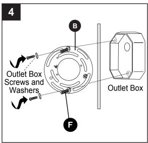
Temporarily place fixture (A) over mounting plate (B) to determine amount of adjustment necessary for screws (F). NOTE: The screws (F) should come through holes in fixture (A) just enough so decorative nuts (D) will fit flush against fixture (A) when mounted.
