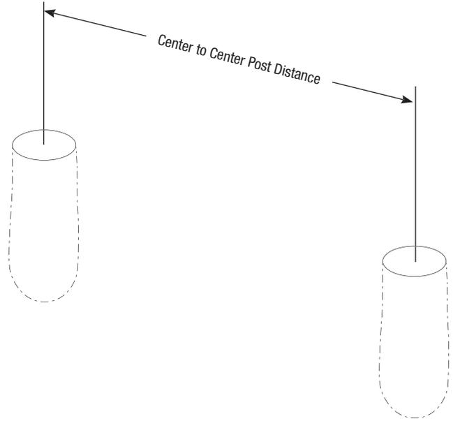
**3a** If frost line does not exceed 30", put 6" of gravel into bottom of both holes and insert posts. Add concrete to first post hole according to manufacturer's instructions to the top of the post hole. Ensure first post is plumb and level. Do not add concrete to second hole until later in installation. Go to Step 4.
