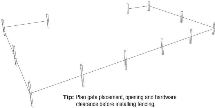
**NOTE:** DO NOT pre-dig all post holes. To ensure proper post spacing, install post-panel-post-panel-etc. until all fence panels and posts have been installed.
