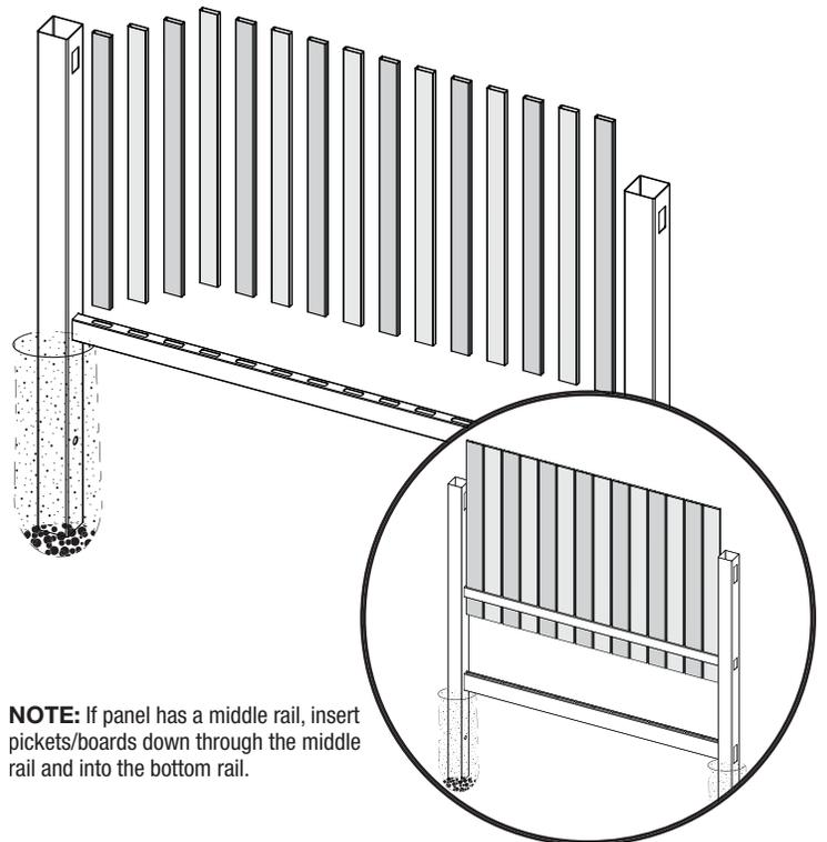
**NOTE:** If panel has a middle rail, insert pickets/boards down through the middle rail and into the bottom rail.
