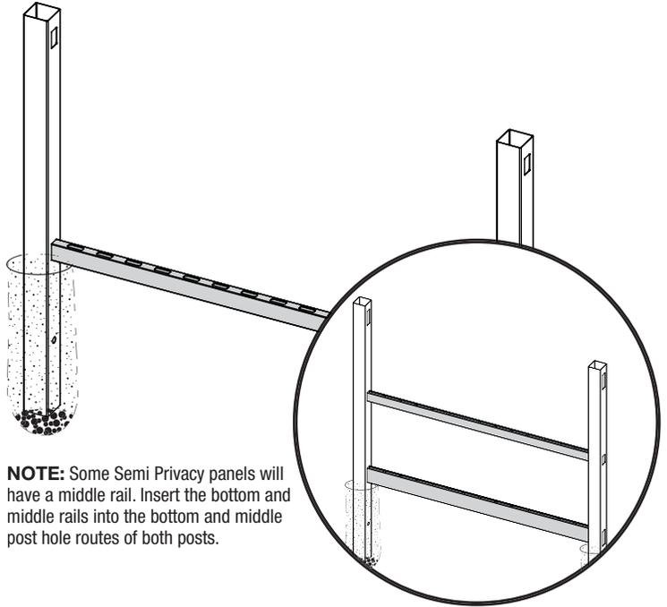
**NOTE:** Some Semi Privacy panels will have a middle rail. Insert the bottom and middle rails into the bottom and middle post hole routes of both posts.
