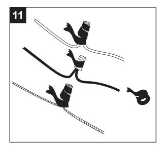
12. Turn the spliced/taped wires upward and gently push the wires and wire connectors (AA) into the outlet box.
