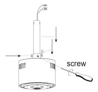
(3) Install in order the yoke cover, Canopy, Hanging Ball on the installed Down rod. slide Hanging Ball down to expose the hole, put the fixing pin into the hole, slide the Hanging Ball up and turn it left and right, let the fixing pin enter the Hanging Ball card slot.
