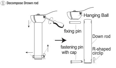
Step 1(Basic assembly of the fan)
