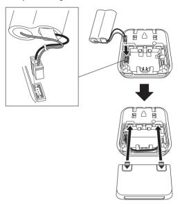
•The battery harness plug has a large notch on it that faces to the left away from the Gas Alarm when installed correctly. There is only one way in which the plug can be installed. A small portion of the plug will be exposed when connected properly.
