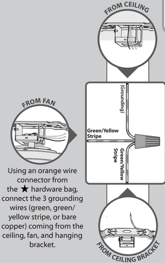
Using an orange wire connector from the ★ hardware bag, connect the 3 grounding wires (green, green/yellow stripe, or bare copper) coming from the ceiling, fan, and hanging bracket.
