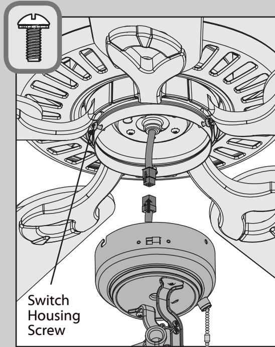
Partially install two of the switch housing screws found in the
