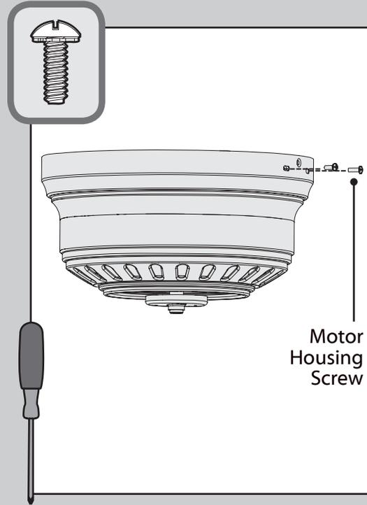
⊗ With a Phillips head screwdriver, install the four motor housing screws found in the ● hardware bag. Tighten all four screws securely.
