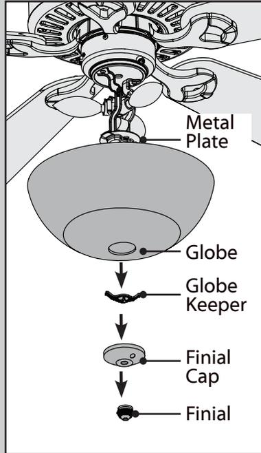
**Changing the bulbs** - unscrew the finial and remove it from the threaded rod. Remove the finial cap and unscrew the globe keeper while supporting the globe with your other hand. Carefully remove the globe. Unscrew bulbs and replace with bulbs of same type and wattage. Reinstall the globe assembly.
