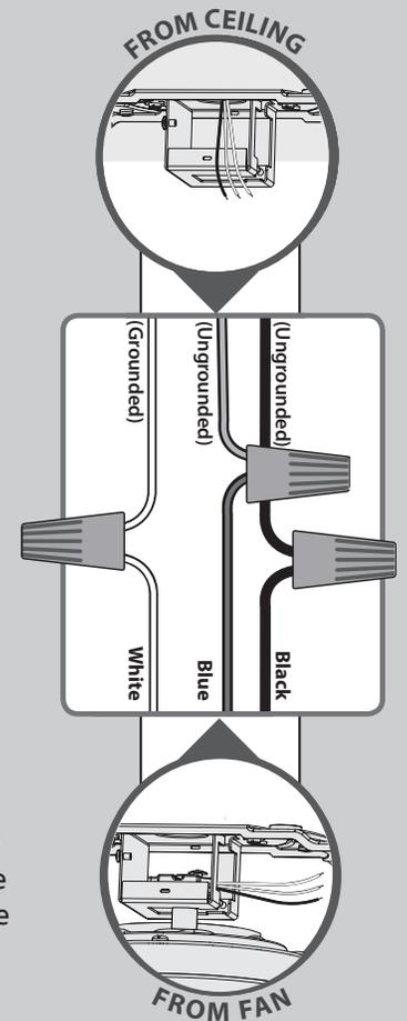
Turn the splices upward and push them carefully back through the hanger bracket into the outlet box. Spread the wires apart, with the grounded wires on one side of the outlet box and the ungrounded wires on the other side of the outlet box.
