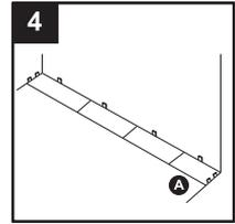
5. Begin the second row with the cut piece (A) from the first row. If the cut piece is shorter than 8 in., do not use it. Instead, begin with a new board that exceeds 8 in. in length and allows 6 in. spacing between the end joints.
