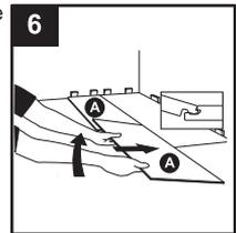
7. Once the ends align, carefully push the second plank (A) of the second row down until its tongue locks with the groove on the first plank (A) of the second row. **Note:** A slight tap with a tapping block (not included) may be necessary to complete interlock.
