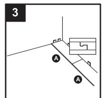
4. Continue in this manner until the first row is complete. Cut the final plank (A) to length, allowing for 1/2 in. expansion space. Place wedges as needed.
