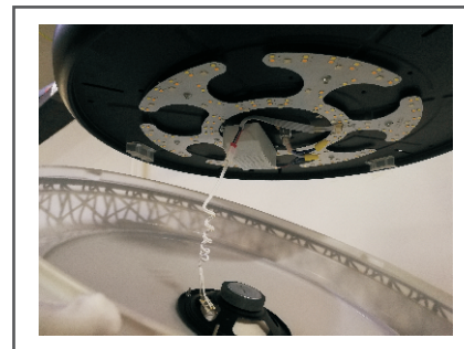
Step 4. Connect the seven-color bluetooth driver cable on the lampshade with the seven-color bluetooth driver cable on the chassis of the fan lamp host.
