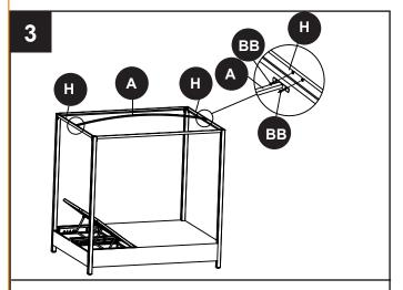
Once all bolts have been installed and hand tightened, go back and tighten firmly.
