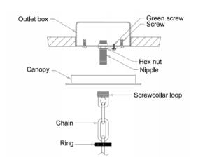
6. Fasten the ground wire to the green or bare copper wire in the outlet box or to the green screw on the crossbar.
