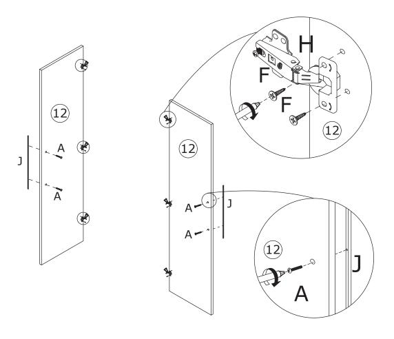
Fix hinge(H) to two plate #12 using screw(F) as shown. Fix handle(J) with screw(A) as shown.
