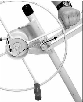
12. Feed the crimped end of the cable through the hole in the winch drum and secure it behind the mooring tab by hand pulling the cable snug as shown.
