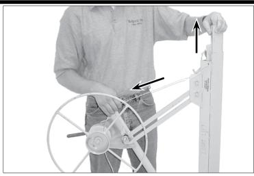
2. Pinch the two telescoping sections together and lift them out as a unit. Pulling the cable will help to raise them.
