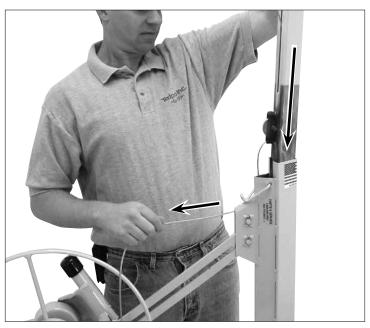
6. Pull the slack cable through the sheave pocket and slide the telescoping sections into the frame housing.
