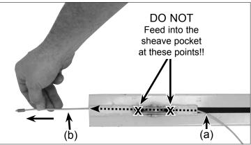
7. Feed the crimped end of the cable down into the slot (a) of the "B" section and out the bottom end of the telescoping section (b) as shown. Pull the cable completely through to remove the slack.
