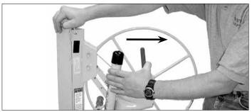
5. Place your right hand on top of the frame and pull the winch assembly towards you. While pulling the winch towards you, grip the brake arm sufficiently to prevent back-lash of the cable on the winch.
