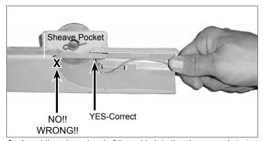
6a. Insert the crimped end of the cable into the sheave pocket at the end nearest the end of the "B" section as shown.
