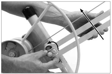
5. Raise up on the slide bar with your left hand while rotating the slide bar lock counter-clockwise with your right hand.
