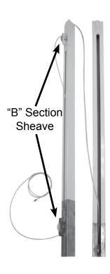
Inspect and replace sheaves (pulleys) before replacing the cable. There are 3 sheaves on the 138-2 Panellift®, one on the frame and two on the "B" telescoping section. Sheaves should be solid on their axle and not move up and down or back and forth. To replace, remove cotter keys and discard old axle and sheave. Replace with new sheave, axle and new cotter keys.
