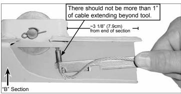
5. Use the special tool provided to insert the crimped end of the cable into the TOP end of the "B" section as shown in this cut away view. On the Model 125 standard "B" section the sheave pocket is located approximately 3 1/8" (~7.9cm) from the end of the section as shown above. On an extended 6' (~182.8cm) telescoping section, wear marks on the section should give an indication of which end is the top.
