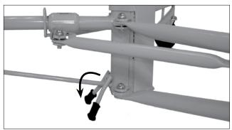
2c. To hold the tripod base in position during this procedure set the backstop as shown.
