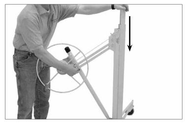
6. While holding the slide bar lock in this disengaged position with your right hand, push down on top of the telescoping section with your left hand. This action will cause the winch assembly to move toward the frame.
