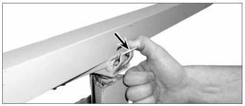
8. Mount the cradle on top of the telescoping section. Flip out the tilt latch to allow the cradle to tilt for loading and for hanging drywall on sidewalls and sloped ceilings.
