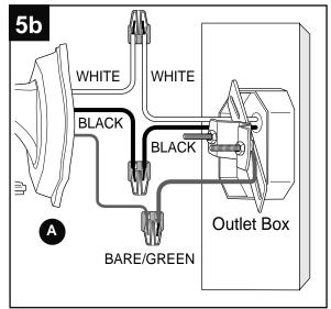
6. Wrap electrical tape (not included) around each individual quick connect clip down to the wire.
