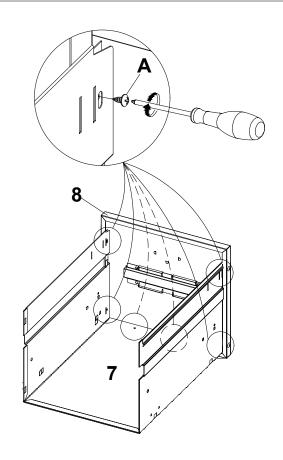
put six screws to hold part 8 into place.
