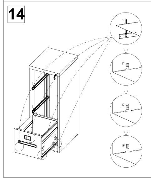
1.pill out the small rails in the slide rails on the side walls completely. with two people lifing each side of the drawer, align the four divots on the bottom with the two rail clips on the rails on each side and insert them into the rail clips.
