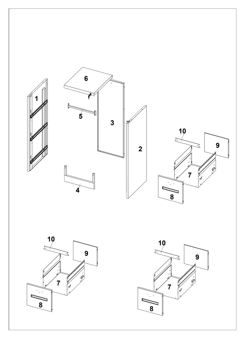
put three screws to hold part 1 and 3 into place.
