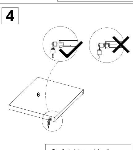
Turn the lock down and place it according to the picture
