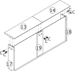
Attach plate 13, 14, 15, 16, 22 and 23 to these components, add cam lock(C) into and turn clockwise to tighten as shown.
