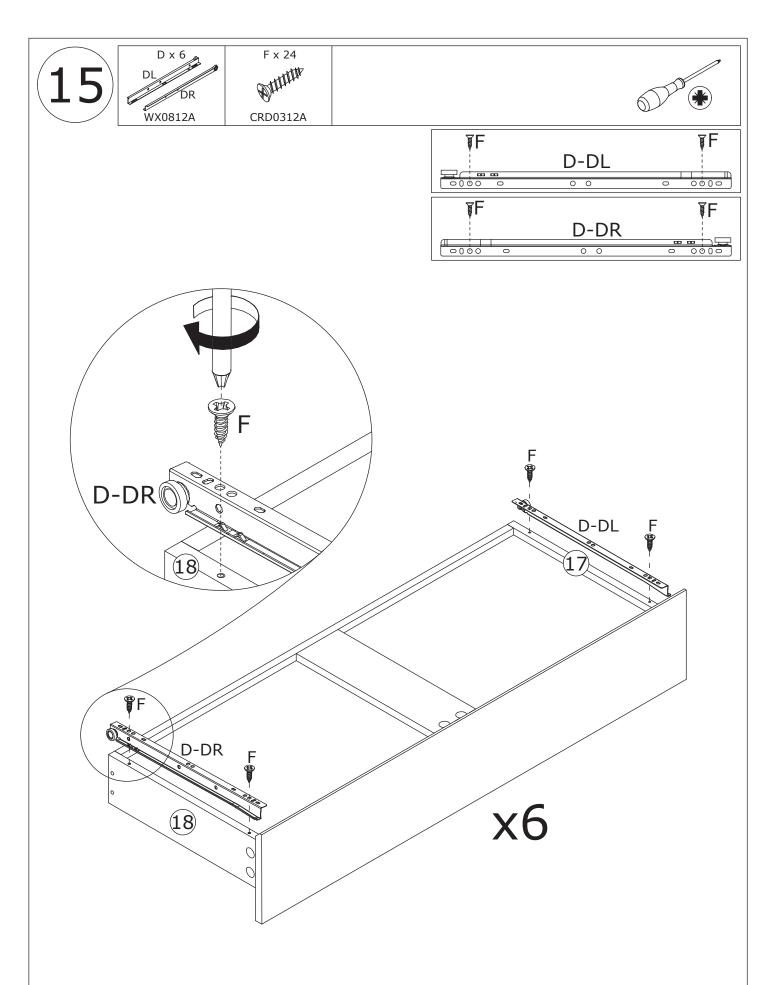
Fix rail(DL) and (DR) to plate 17 and 18 with screw(F) at first.
