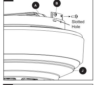
2. Slide the motor housing (J) over the motor (D), aligning the slotted holes in the motor housing (J) with the loosened motor housing screws (B) in the upper mounting bracket (A). Twist the motor housing (J) to lock, then re-insert the two previously removed motor housing screws (B) and securely tighten all screws.
