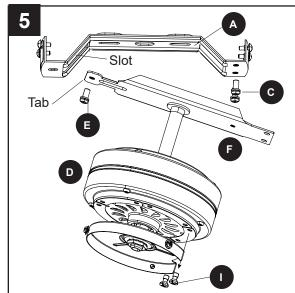
6. Re-install the previously removed lower bracket screw (E) and upper bracket screws (C) to secure the lower mounting bracket (F) to the upper mounting bracket (A).
