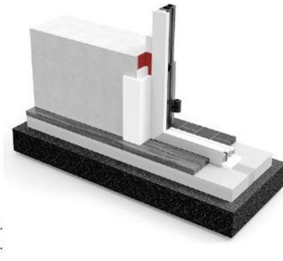
Vapour barrier tape on the inner contour
