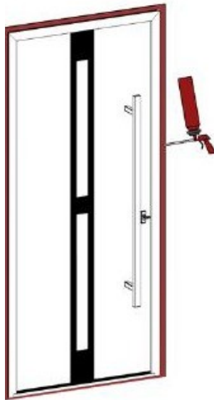
Covering the frame fixing openings with the supplied caps
