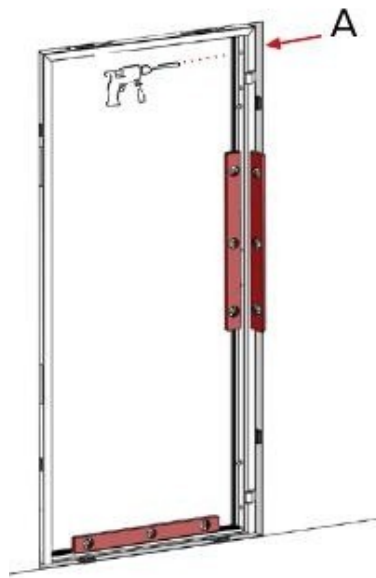
Drilling through the upper mounting hole on the hinge side
